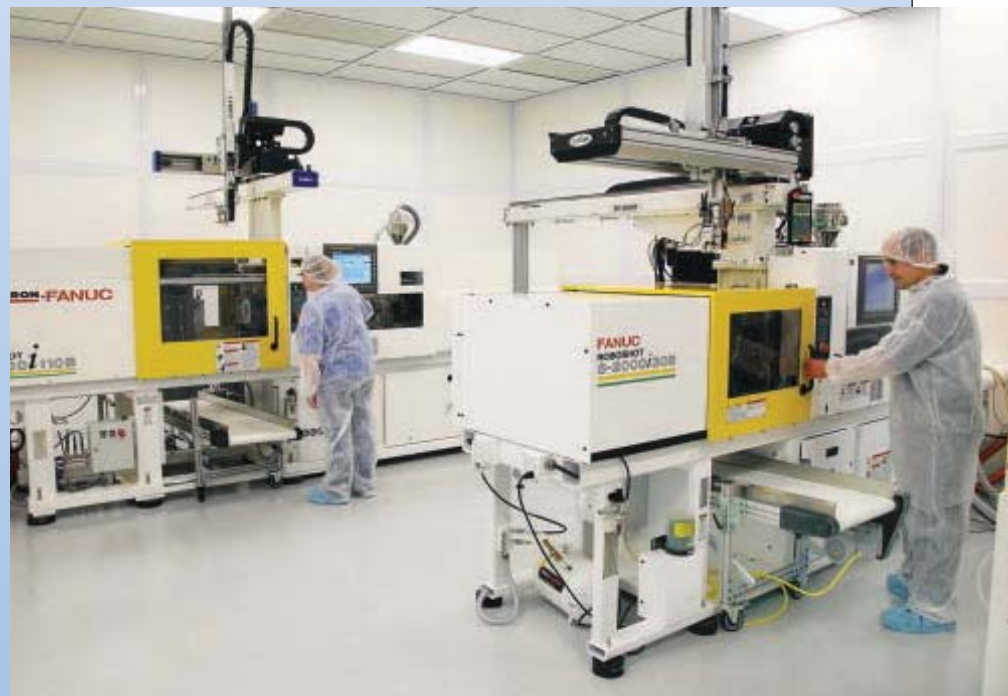
▲ PMC's fleet of Roboshot machines enables ultra-precise molding in the company's Class 100,000 cleanroom.
